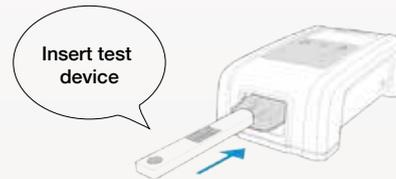
**Step 2.** Open the aluminium test pouch and insert the LifeAssays® test strip into the Reader (small arrow on the end of the test device is visible and pointing towards you). The sample well marked with “S” will remain outside the Reader.
