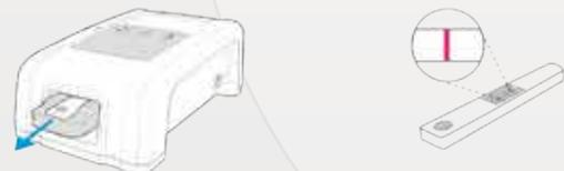
**Step 6.** After recording the result, remove the LifeAssays® test device from the Reader and check the control line visually. A pink control line in window area next to the letter “C” appears. If there is no control line, the test result is invalid and should be discarded.
