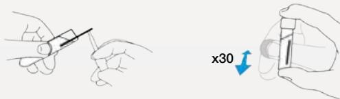
**Step 3.** Collect the serum/plasma sample using the 5µl glass capillary and fill completely. Wipe off excess fluid with a clean tissue. Place the capillary into a buffer vial and mix by inverting the tube at least 30 times.
